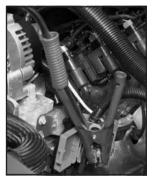
The remote positive (+) terminal is located near the engine accessory drive bracket. On some vehicles, the terminal may be covered under under a red plastic cover. To access the remote positive (+) terminal, open the red plastic cover.
